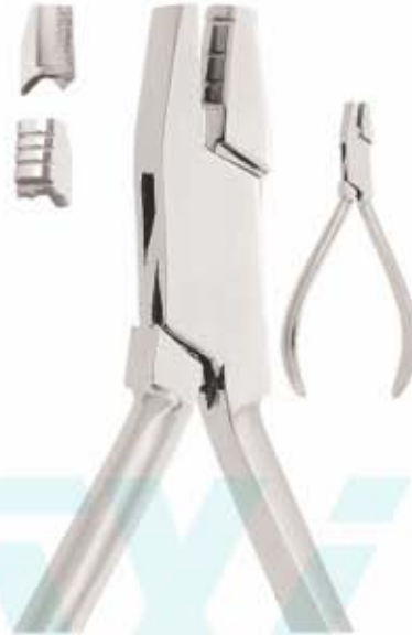
TW5-58 Arch Counting Plier Grooved for double back and triple back bands in 0.30" / 0.76mm & 0.36" / 0.91mm lingual arch wires 135mm
